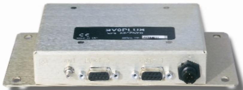
The SV8PLUS receives satellite signals, calculates its location on Earth, and outputs a data stream to a Campbell Scientific datalogger.
