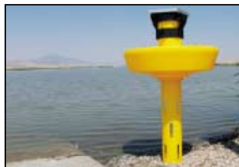
Completely self-contained, the CSBUOY measures water quality parameters in fresh water.
