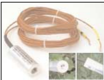
Automate leaf and soil surface temperature measurements using the compact IRTS-P. (Inset photos show recessed lens and mount.)
