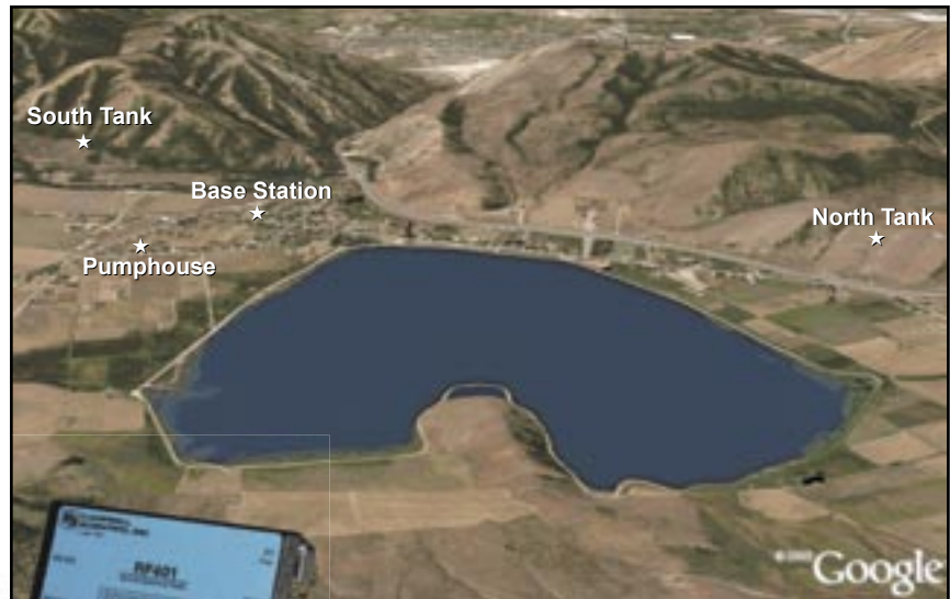
PAKBUS®-based radio networks, such as those that use the RF401, can telemeter data from remote sites to a central base station. Shown is a rural water network.
