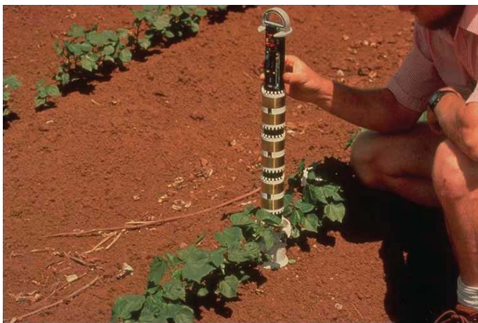
The EnviroSMART is inserted into an access tube in a row of cotton.
