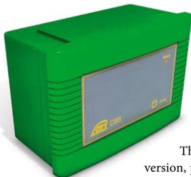
The CS470 and CS471 determine liquid level by measuring the pressure required to force compressed-air bubbles through a submerged tube. A pressure transducer measures the tube pressure and the atmospheric pressure at the surface. This technique compensates for temperature effects and long-term drift in the transducer, producing a more accurate measurement.
