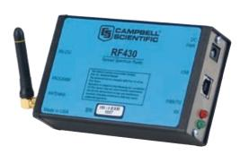
To make it easier to connect to newer computers, we are releasing three new spread-spectrum radios with USB ports. The new RF430 (900-MHz), RF431 (922-MHz), and RF432 (2.4-GHz) radios are functionally the same as our RF401 series. The difference between the two is that the RF430 series has both USB and RS-232 ports, while the RF401 series has RS-232 and CS I/O ports.
