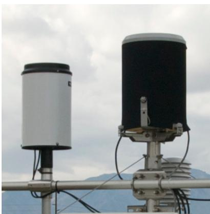
Campbell Scientific now offers the 52202 and CS700H heated rain gages. The 52202 is manufactured by R.M. Young and is intended for standard applications. It measures precipitation in 0.004-in. increments, with an accuracy of 3 percent for up to 2 in./hr.
