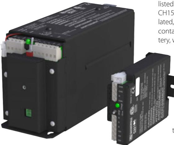
Campbell Scientific offers two new ETL listed Class 2 power supplies, the PS150 and CH150, for recharging 12 Vdc, valve-regulated, lead-acid (VRLA) batteries. The PS150 contains a 12 Vdc, 7 Ah rechargeable battery, whereas the CH150 is for applications where the user provides the battery, such as our BP12 or BP24.
