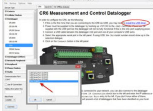
Then connect your computer to the CR6 using the supplied USB cable from the bottom compartment of the CR6 box. Now, the USB communications port will show up in the selection list as CR6 (COM number).
