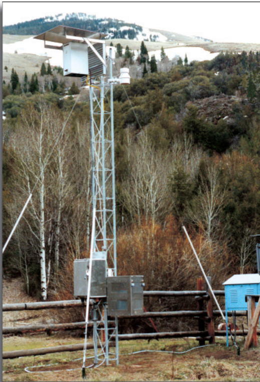
This station, located in the Jarbridge Wilderness Area in Nevada, measures visibility as part of a long-term study to protect scenic views in U.S. parks and wildernesses.
