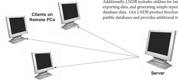
Clients running on remote PCs use TCP/IP to connect to the server of the Datalogger Support Software. For each remote PC, one copy of the client software must be purchased.
