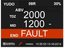
The controller, which can be mounted in a 19" rack or be positioned on a desktop, also accepts input from the runway lighting system to provide the runway light intensity (RLI) and an input to determine the operational direction of the runway (RD). Using a combination of visibility and background luminance sensors in conjunction with the RLI and RD, RVR can be calculated for each deployed runway location in accordance with ICAO standards.
