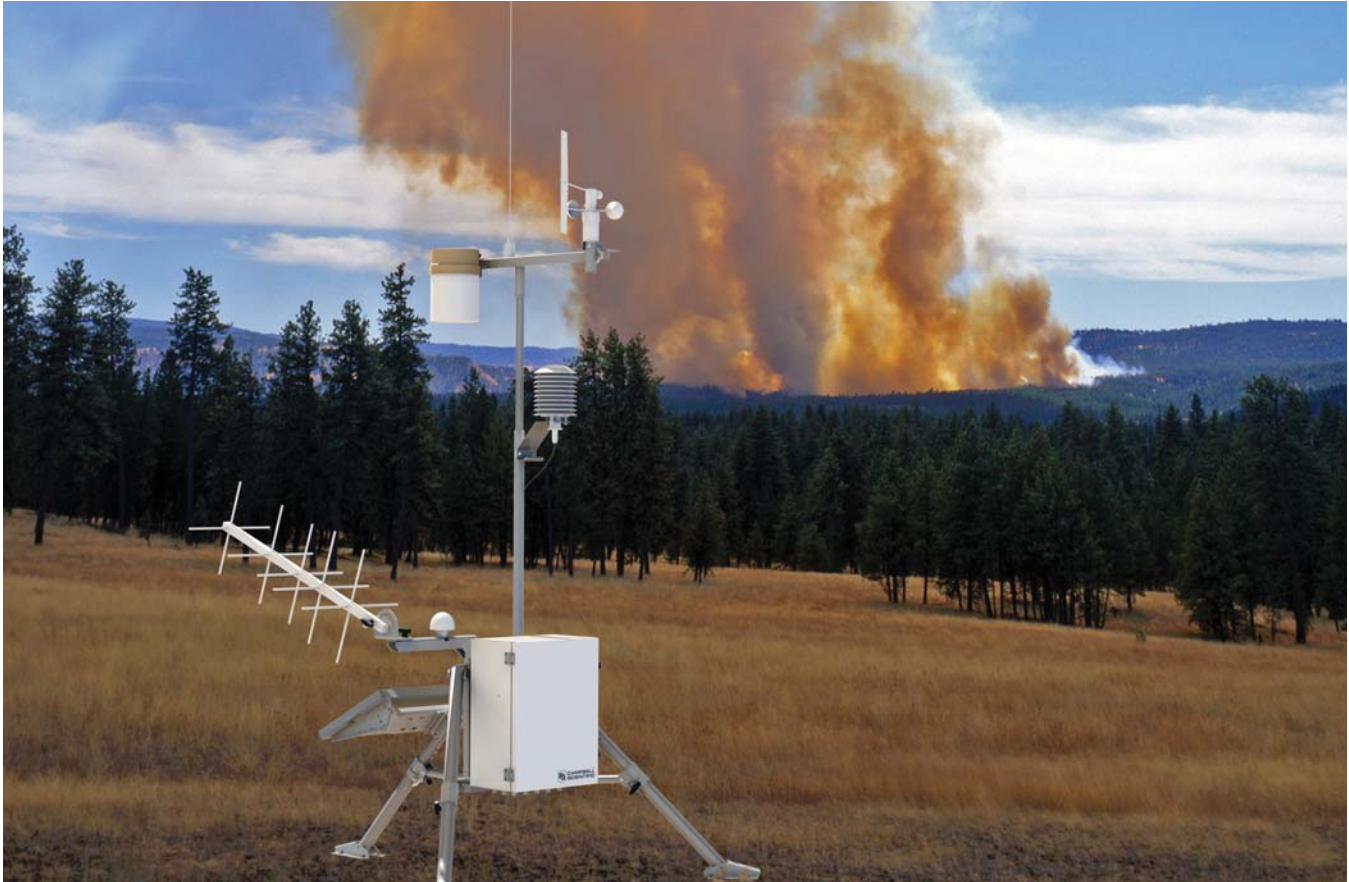
Meteorological sensors included with the RAWS-F are the CS300-QD Solar Radiation Sensor, HC253-QD Air Temperature and Relative Humidity Probe, TE525-QD Tipping Bucket Rain Gage, and either the WindSonic4-QD 2-D Sonic Wind Sensor (not shown), or 034B-QD Wind Set.
