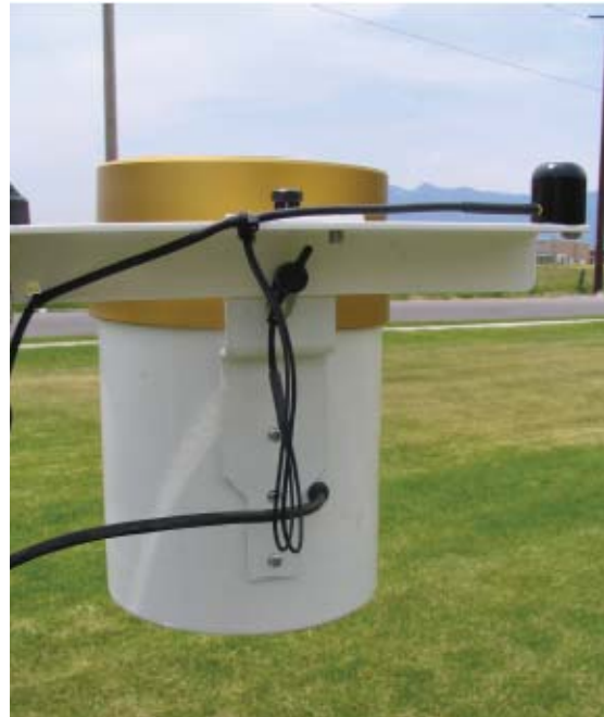
This view shows the TE525-QD tipping bucket rain gage and the CS300-QD pyranometer (right).
