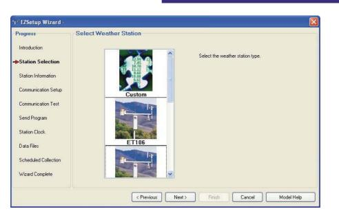
The Visual Weather EZSetup Wizard helps you easily configure a weather station for communications, data collection and report generation.
