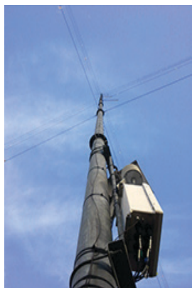
A datalogger based system mounted on a met mast Image courtesy of Meteoright
