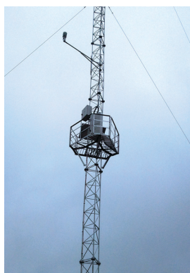
Sensors are mounted at various points up to hub height Image courtesy of Lufft GmbH
