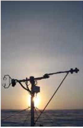
*Measuring CO<sub>2</sub> and H<sub>2</sub>O fluxes with open or closed-path Eddy Covariance systems.*
