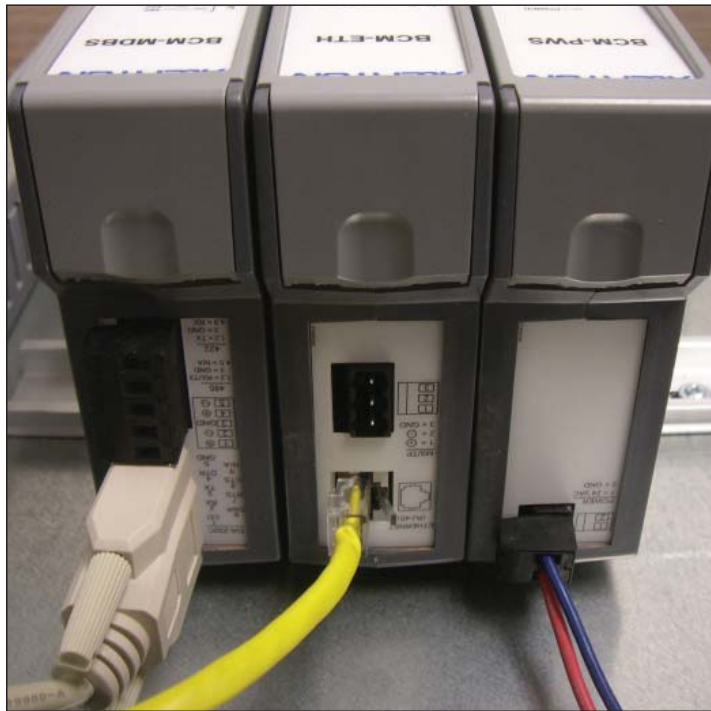
Figure 4: At bottom left, the SC110's DB9 female connector is attached to the BCM-MDBS. At center, a yellow Ethernet cable is connected to the Ethernet port on the BCM-ETH. The BCM-PWS connects to a 24 Vac source.
