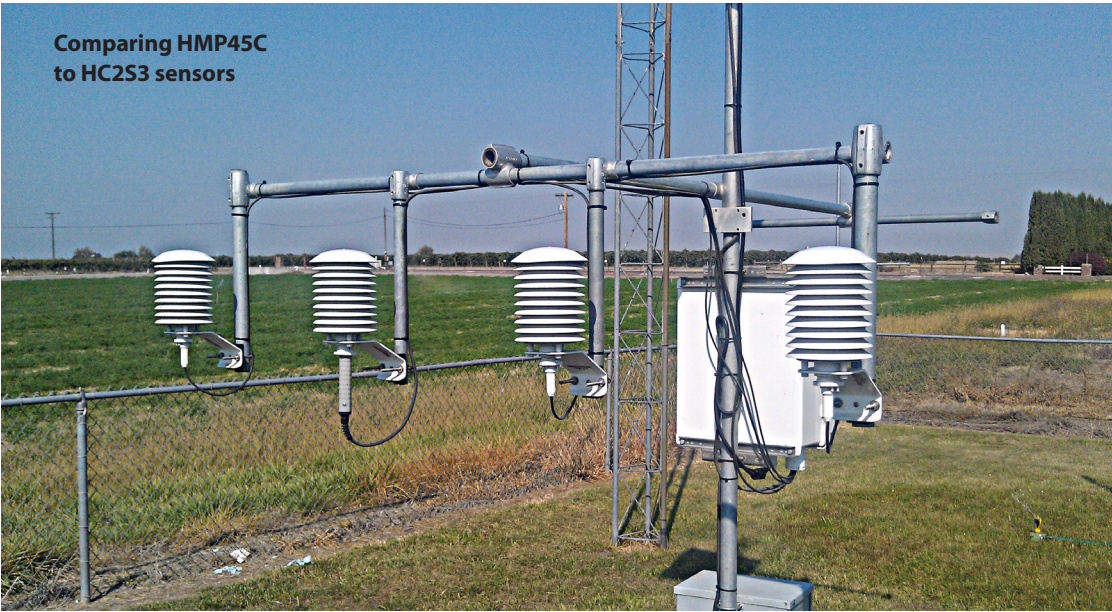
Comparison array testing 107-L temperature sensors
