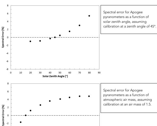
Spectral error for Apogee pyranometers as a function of atmospheric air mass, assuming calibration at an air mass of 1.5.
