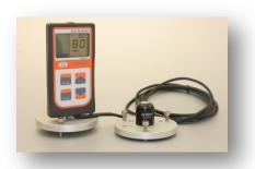
The AL-100 leveling plate is recommended for use with the MP-200. To facilitate mounting to a cross arm, the AM-110 mounting bracket is recommended for use with the AL-100.
