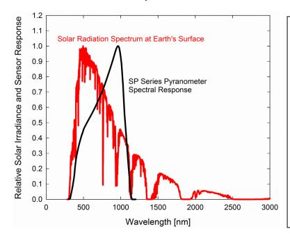
Spectral response of Apogee silicon-cell pyranometers compared to solar radiation spectrum at Earth's surface.
