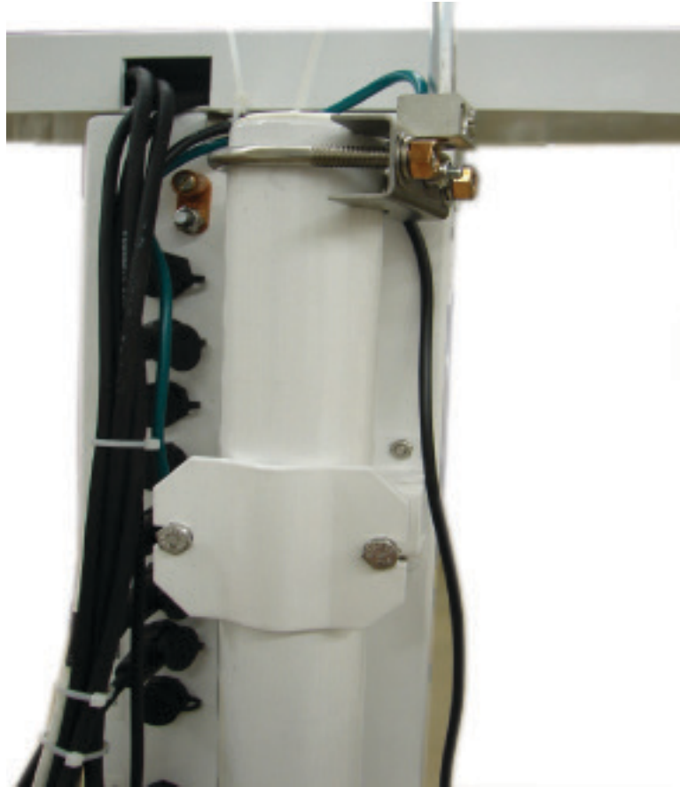
FIGURE 2-30. Loosely Drape Antenna Cable over Back of Enclosure
