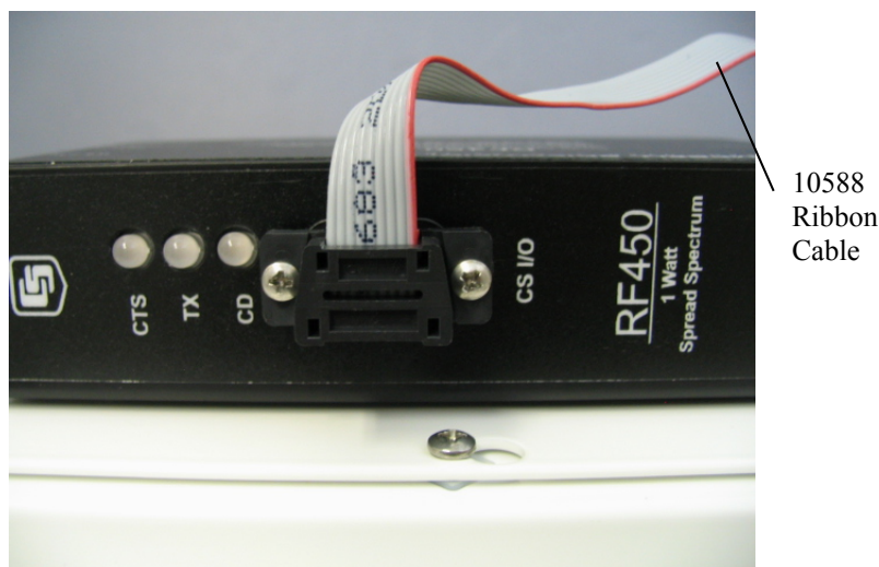
FIGURE 2-28. Attach Ribbon Cable to RF450 CS I/O Port
