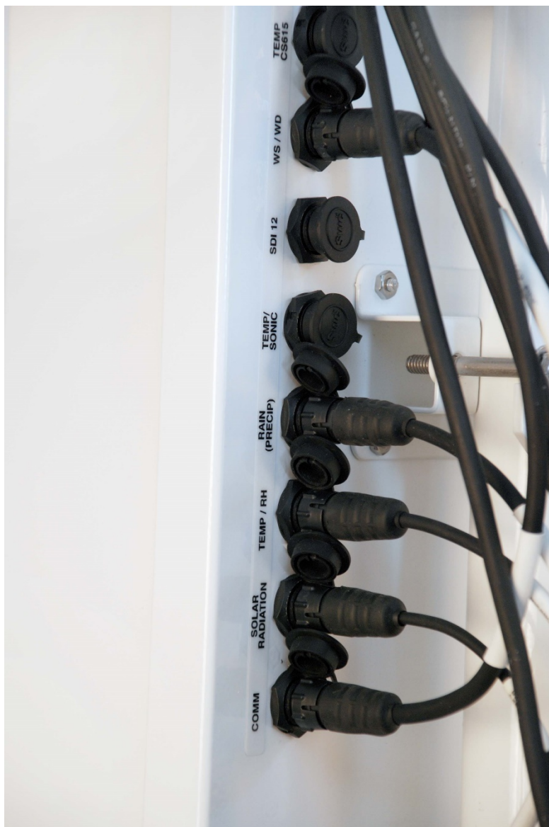
FIGURE 2-22. Connecting Sensor Cabling to Enclosure
