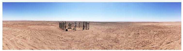
In addition to the meteorological measurements, Valhalla also calculates a solar-panel soiling index based on short-circuit current measurements from a solar panel that is maintained clean, and one that is left to the elements.
