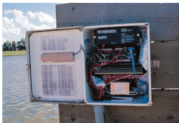
Though pond-condition data can be viewed and controlled via a personal computer, special display-equipped enclosures (shown open above) also make data visible on-site.
