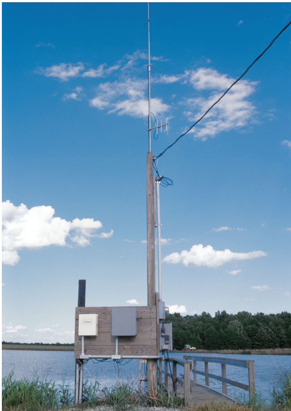
A Campbell Scientific CR10X Monitoring and Control system eliminates the need to manually check DO concentrations several times a night. Alarms are sent via RF to a computer.
