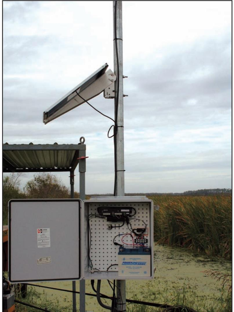
*A CR510 datalogger routinely measures water level and rainfall at a standard field site.*
