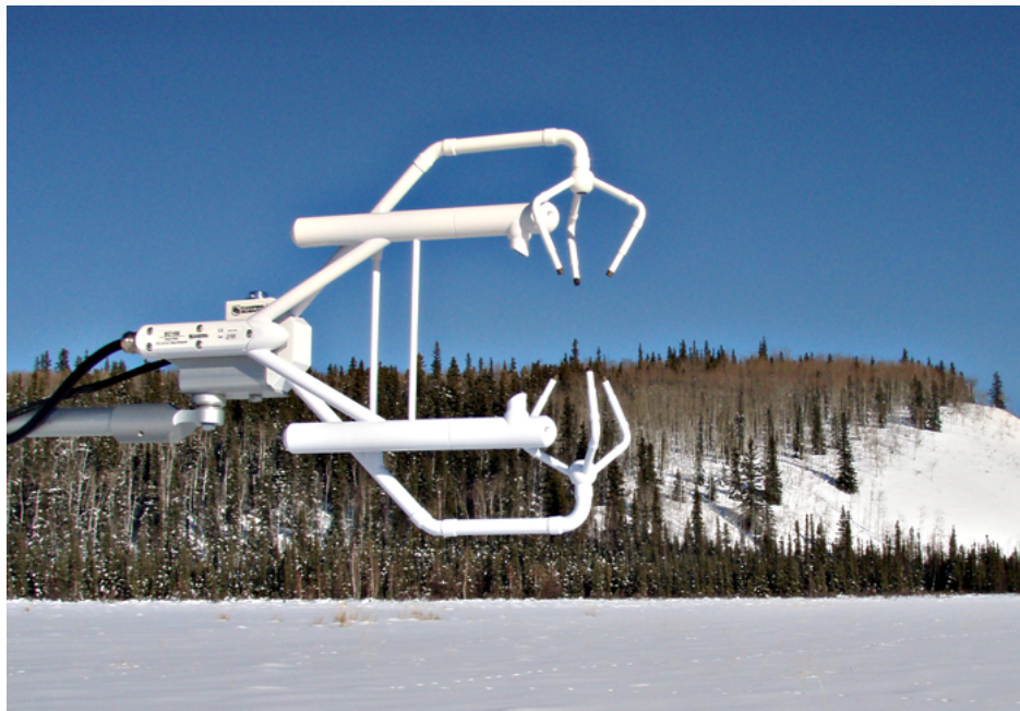
EC150 open-path CO 2 /H 2 O analyzer with CSAT3A sonic anemometer at a Bonanza Creek site
