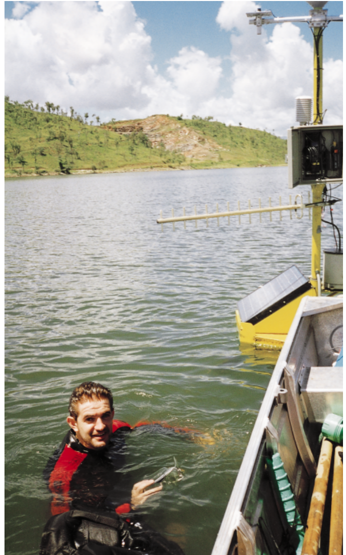
Campbell Scientific Australia's Chris Kellet installs the underwater thermistor chain on Ross River Dam's weather station.
