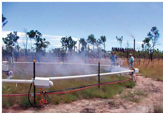
Testing the CO 2 delivery system with a smoke generator during the OzFace installation.
