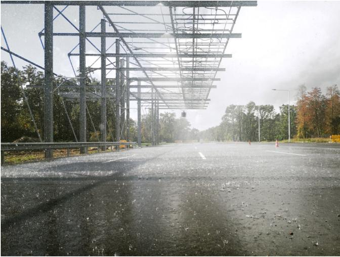
*The outdoor rain plant on the test track
