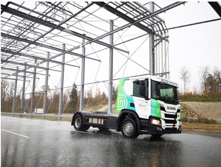
A truck testing the outdoor rain plant on the test track
