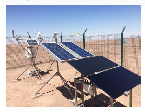
Valhalla, an energy company in Chile, is making resource assessment and solar-panel soiling measurements in advance of construction of the Cielos de Tarapacá Project.
