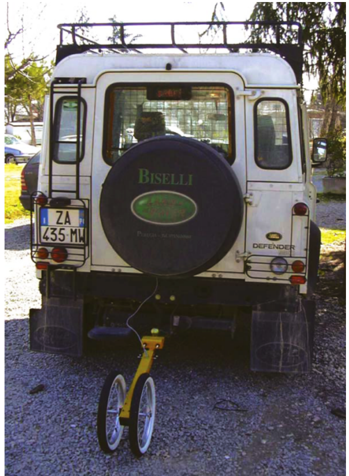
An odometer fitted to one of the road-map vehicles in the Perugia, Italy, road ice project, makes precise measurements of distance traveled.
