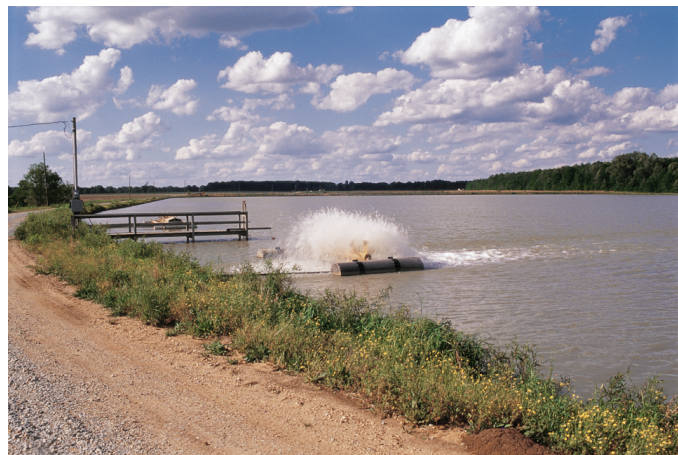
An automated aerator restores dissolved oxygen levels on one of many ponds at the Lee Catfish Farm in Mississippi. In addition to water conditions, current drawn by the aerator can also be monitored.
