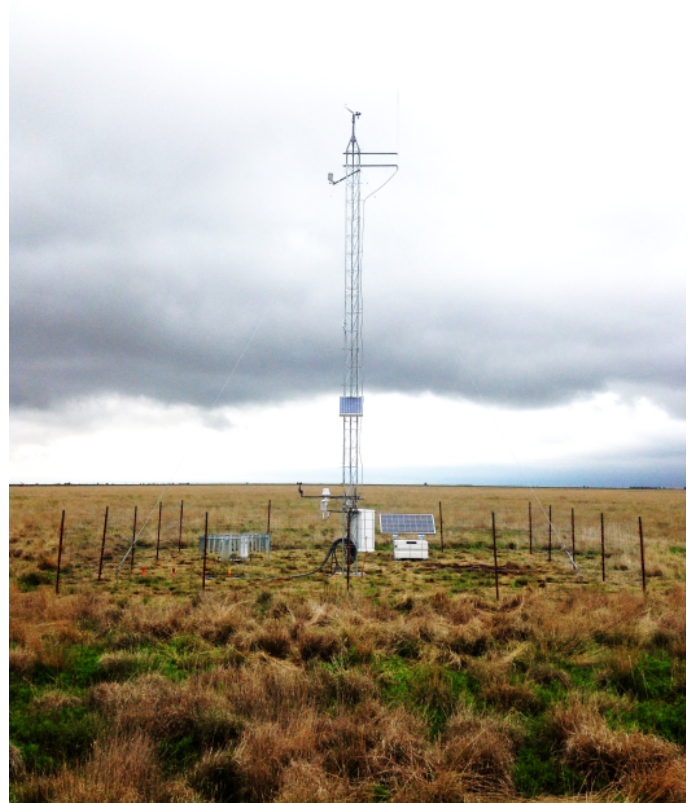
A mesonet station at Eufaula, Oklahoma, is one of 121 automated weather stations that continuously measure weather conditions.
