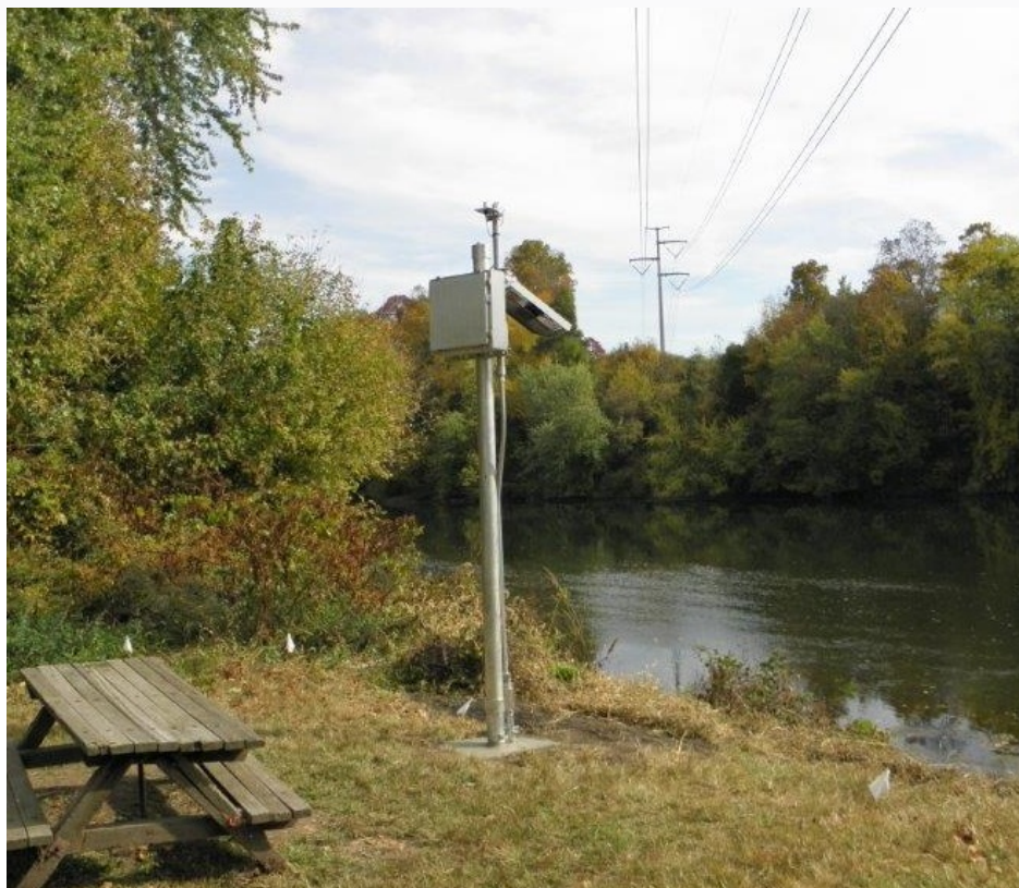
Campbell Scientific system monitoring river level
