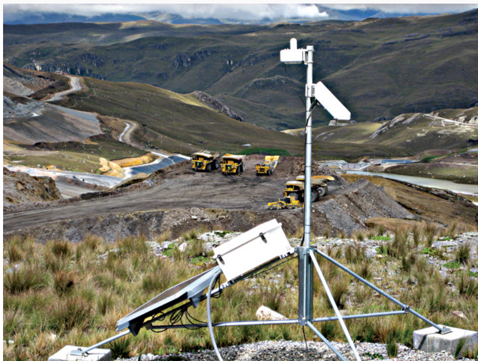
Warning system with CS110 Electric Field Meter
