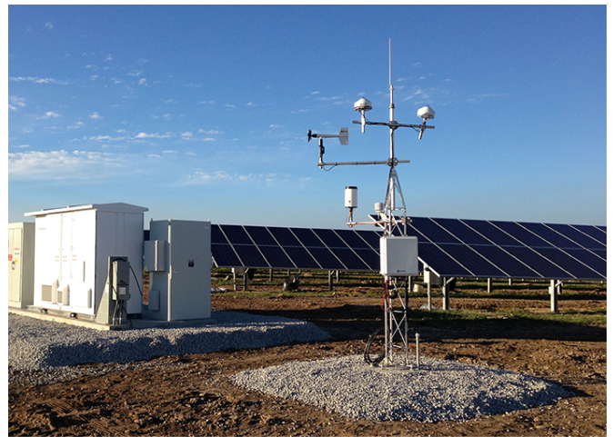
An automated weather station for solar farm performance monitoring. This turnkey system was customized by Campbell Scientific to meet the specific requirements for Ontario solar farms.
