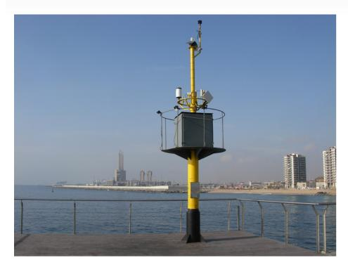
The tower provides measurements of meteorological parameters plus sea conditions for scientific research but also provide useful information for users of the beach.
