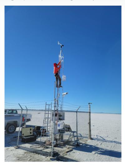
The Utah Geological Survey, supported by the Utah Division of Water Rights, has constructed a network of eddy-covariance stations across Utah to measure evapotranspiration. These stations measure the combined water evaporation from land and water transpiration by plants. Consumptive use—the water absorbed and transpired by plants—contributes significantly to evapotranspiration in vegetated areas, including croplands.
