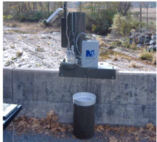
Enclosure ready to install in standpipe
