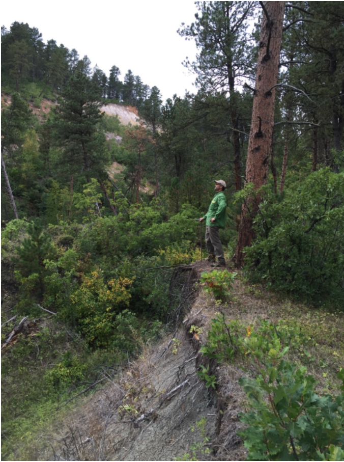
RESPEC geologist conducts reconnaissance along the landslide's inner scarp valley for drilling road access. The head scarp is visible in the background exposing mudstone of the Jurassic Morrison Formation.
