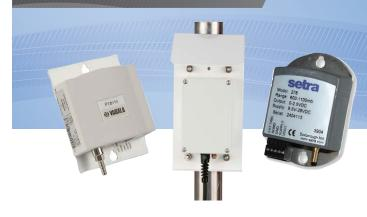
Barometric pressure sensors measure fluctuations in the pressure exerted by the atmosphere. The sensors require protection from condensing humidity, precipitation, and water ingress and are typically housed with the datalogger inside an environmental enclosure. If the enclosure is airtight, the sensor's pressure port must be vented to the atmosphere.
