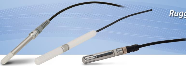
Air temperature and relative humidity probes typically consist of two separate sensors packaged in the same housing. Often relative humidity is measured with a capacitive RH chip, while air temperature is measured by a PRT. The HMP155A, HC253, or CS215 is recommended
