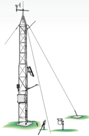
Instrumentation towers are stable structures on which components of data acquisition systems are mounted. Because of their additional height (up to 30 ft), towers allow greater measurement heights than instrument tripods. For easier shipping and on-site installation, instrumentation towers consist of 10 ft sections.
