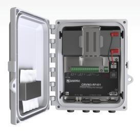
Vibrating wire data loggers have the built-in capability to measure vibrating wire sensors. These data loggers use patented spectral analysis technology.
