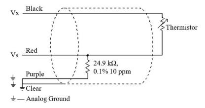
Figure 8-1. 109SS thermistor probe schematic
