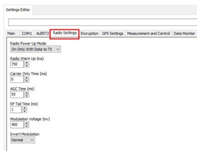
If using a different type of radio, consult the manufacturer to determine the settings. The following are descriptions of the radio settings.
