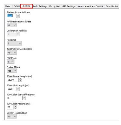
Station Source Address (1000) – This station ID is an integer between 1 and 65,501 that must be unique within the network. Never have the same ID on more than one device in a network, including repeaters and decoders. A database of source addresses can be found at www.alert2.org  $\square$ .
