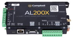
The AL200X includes an RS-232 port for serial communications. A USB device port is used for configuring the AL200X, viewing real time readings and computed values of sensors, and diagnostics. An SMA female connector is provided for connecting a GPS antenna, and a removable connector with screw terminals allows for connecting an analog radio. Removable
