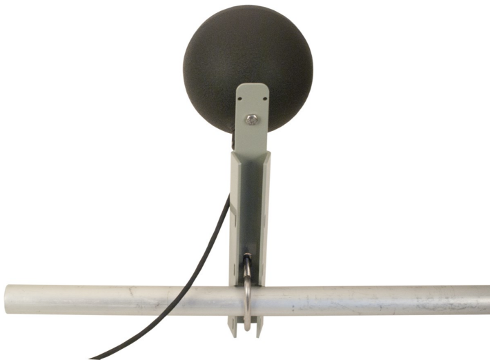
Figure 7-5. BlackGlobe mounted to a crossarm (back view)
