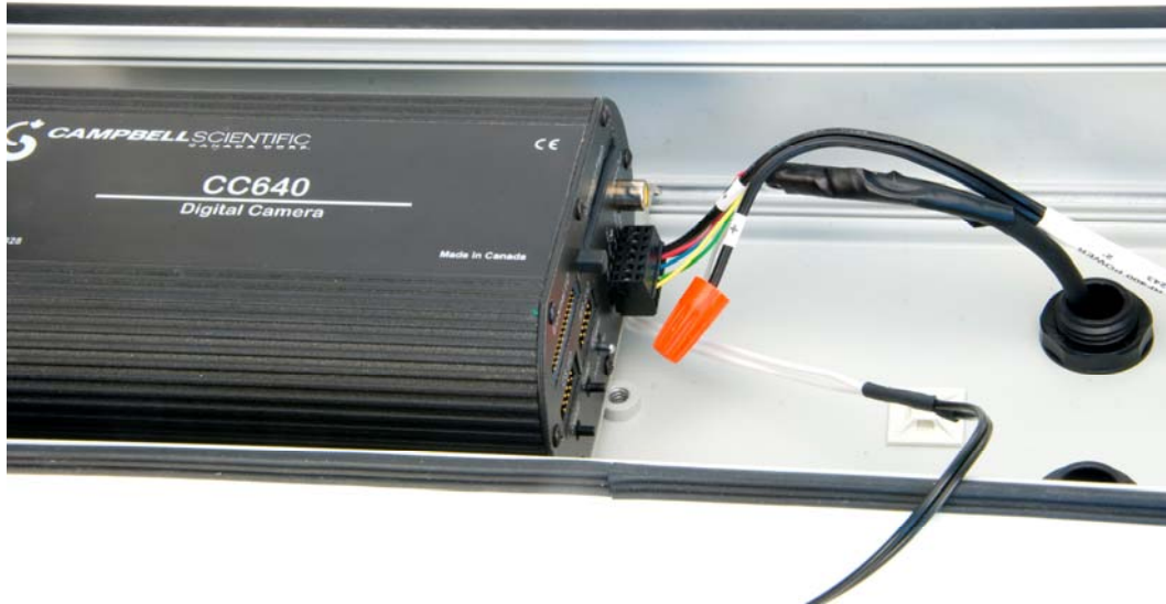
FIGURE B-3. Field Power Cable Connected to the Camera
