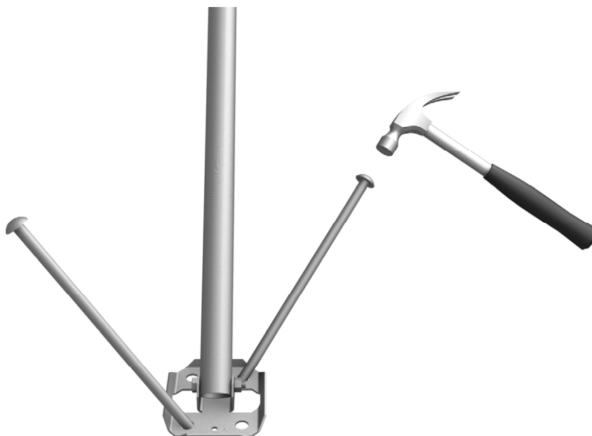
FIGURE 5-7. Staking the tripod feet
