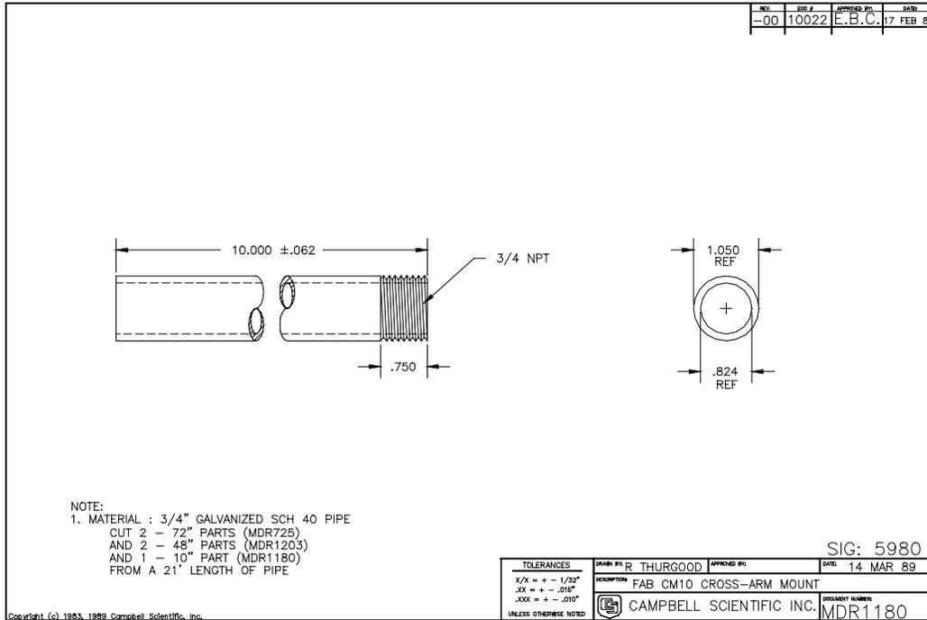
**FIGURE 1-3. CM6 / CM10 Tripod Crossarm Mechanical Drawing**
