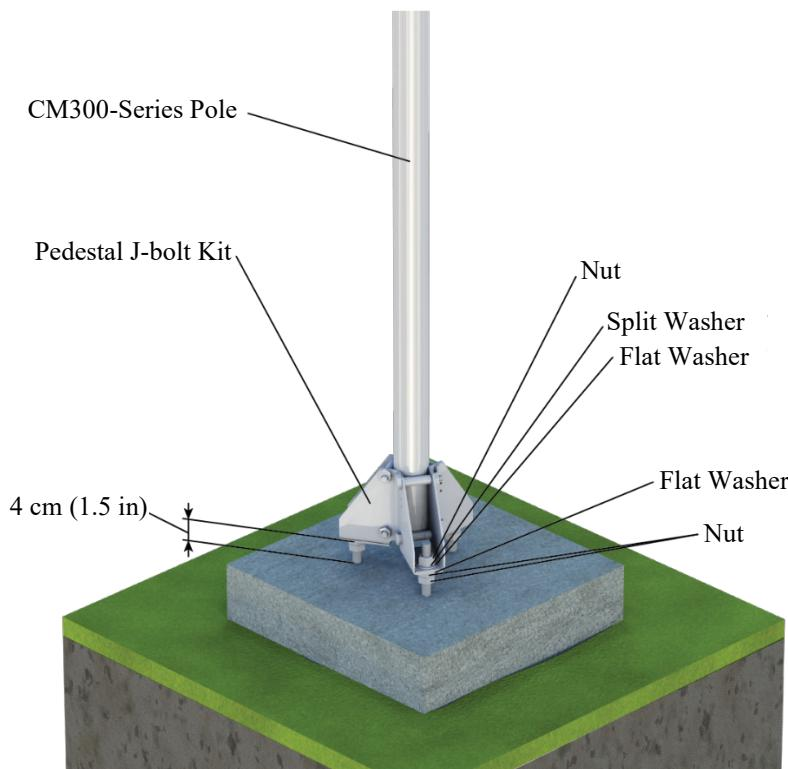
*FIGURE 3-4. CM305 Mounting Pole with Pedestal J-Bolt Kit*
