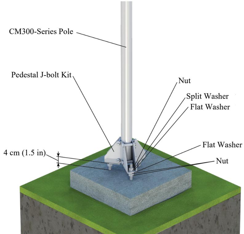
FIGURE 3-4. CM305 Mounting Pole with Pedestal J-Bolt Kit
