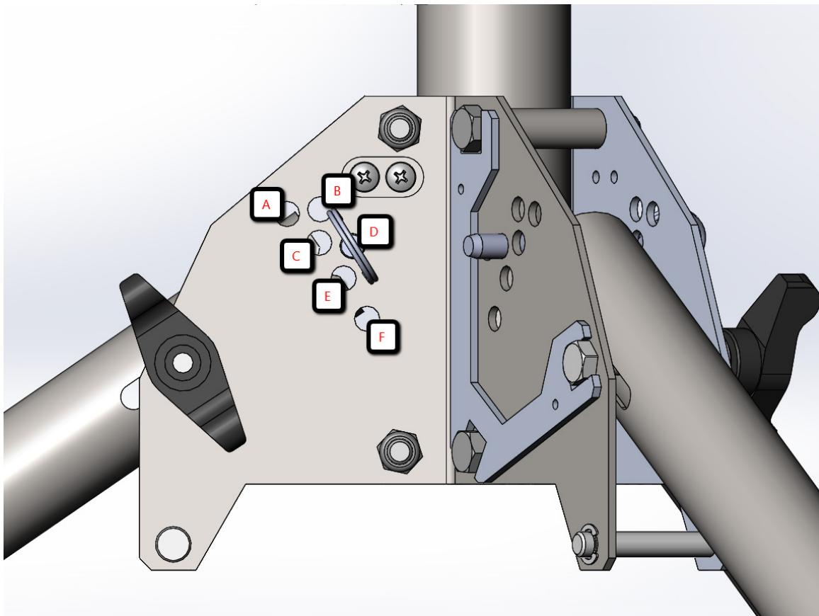
FIGURE 3-5. Pedestal Leg Base Showing Incline Holes
