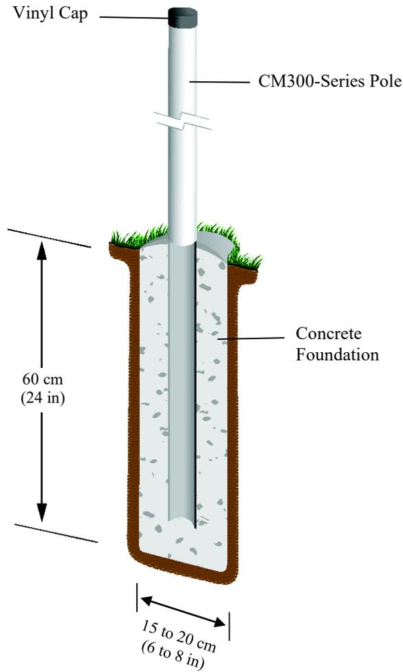
FIGURE 3-1. CM310 Mounting Pole in Concrete Foundation
