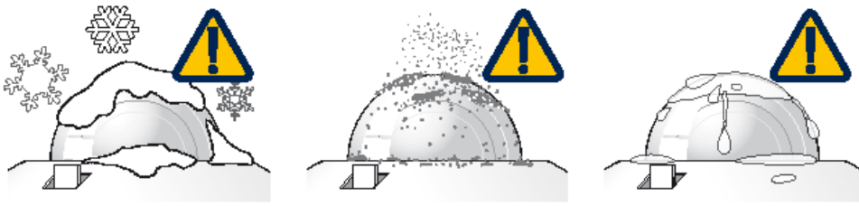
Figure 7-1. Reading is reduced if dome is not dry or clean
