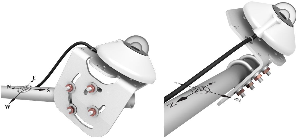
Figure 6-4. Two views of a pyranometer mounted at an angle for the Northern Hemisphere
