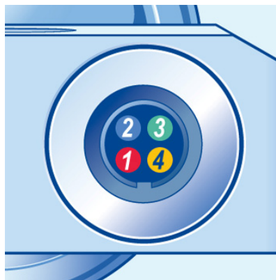
FIGURE 5-2. Pin Layout on Kipp & Zonen Original Cable
